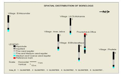
Fig. 3. Striplogs and distribution of borelog location in and around Betagi Paurashava (IWM, 2013)
